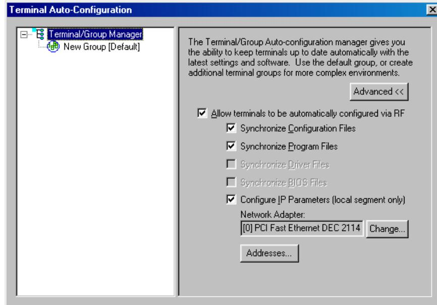
This powerful software management tool is described in detail in the section entitled *Airloader Auto-Configuration*. For now, it is sufficient simply to use it for assignment of the initial terminal configuration and IP address, both of which can be easily changed later. Ensure that all of the check boxes are checked as shown above.
